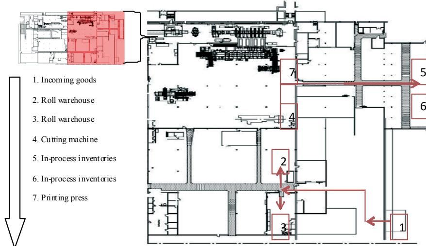
Having reviewed the given material flow for print carriers, we had to admit that neither the location of the in-process inventories, nor the place of the roll warehouse was optimal. The movement of print carriers demanded considerable time and energies due to the considerable distances. The base materials were not available where they were actually needed.
