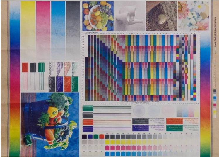
Figure 8: Image of CMYK colour profile test
