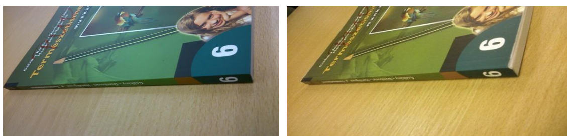
Figure 4: B/5 sized book showing the least abrasion on the spine edges
