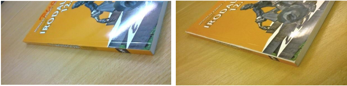
Figure 5: The largest extent of spine edge abrasion has been experienced for B/5 sized book 10-12
