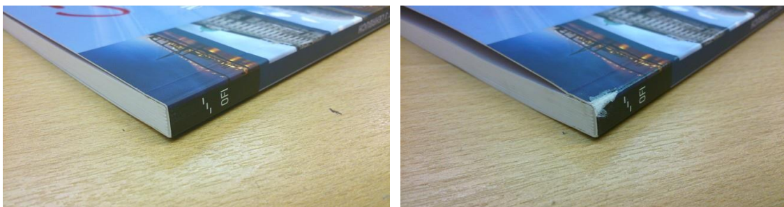
Figure 9: Slight spine corner abrasion on the 28-30 thread-stitched school book
