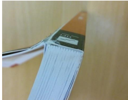
Figure 13: Conditions of binding on the A/4 format, 25-27 thread-stitched school book
