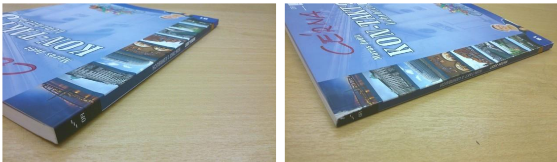
Figure 6: A/4 sized, 28-30 thread-stitched school book with a smaller extent of spine edge abrasion
