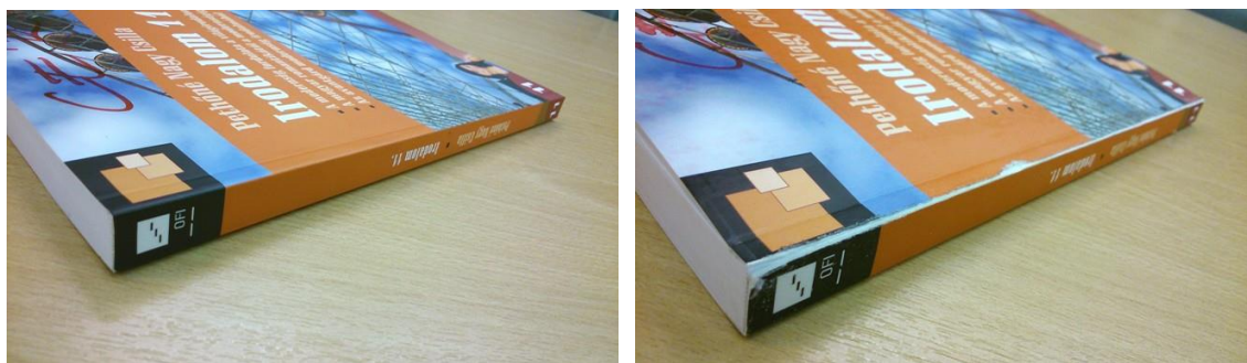
Figure 7: A/4 format, 25-27 thread-stitched school book with a considerable extent of spine edge abrasion
