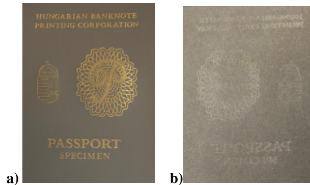
Figure 7: Gilded substrates showing strong deformity on the back. a) front, b) back
